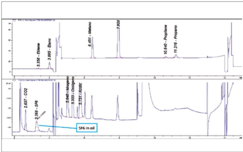
Figure 6. Example of SF<sub>6</sub> detection in DGA, TCD detector, with a switching valve to exclude the methanizer
