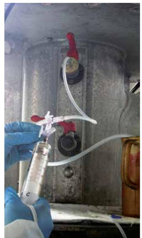
Figure 5. Oil sampling from SOT bushing
