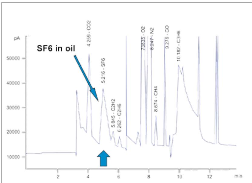
Figure 7. Example of SF<sub>6</sub> detection in DGA, PDD detector
