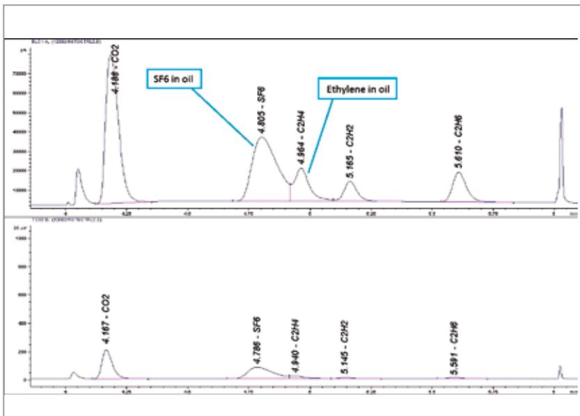
Figure 8. Example of SF<sub>6</sub> detection in DGA (separation from ethylene), PDD detector
